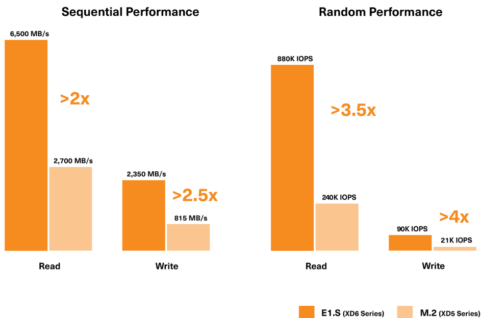
Figure 1: E1.S SSD (XD6 Series) vs M.2 SSD (XD5 Series) performance comparisons
