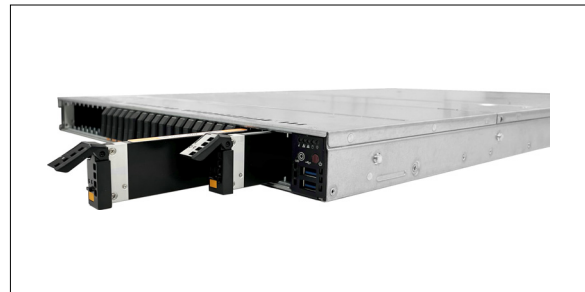
Hot-swap capabilities with KIOXIA XD7P E1.S SSDs
