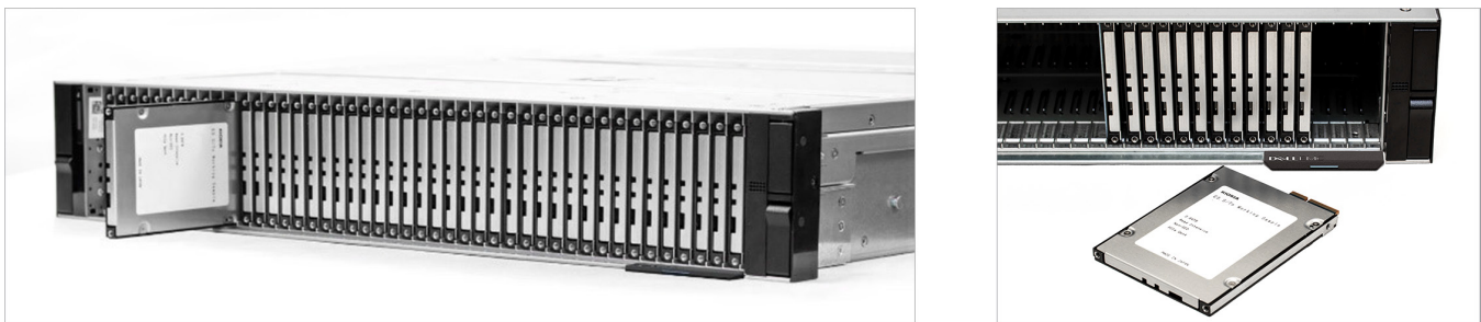
Figure 1: EDSFF prototype with KIOXIA E3.S Prototype NVMe SSDs
