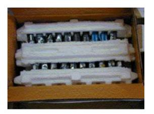
**Examples of <u>UNACCEPTABLE</u>** return packaging. Inadequate physical or electrical protection provided.
