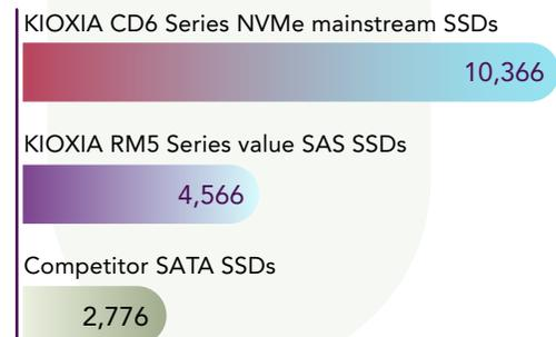
Figure 1: Max throughput in MB per second of a vSAN cluster of three HPE ProLiant DL385 Gen10 Plus servers running Vdbench with a 100 percent sequential read I/O profile using 128k blocks. Higher is better. Source: Principled Technologies.
